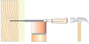
1. Position the tie into the hand held fixing tool as shown above. Drive directly into timber stud through insulation.
