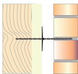
2. Place insulation support over tie, and embed the outer end into the outer leaf mortar.
