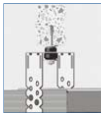
Example of a ceiling fixed to concrete with the SureHit acoustic fixing
