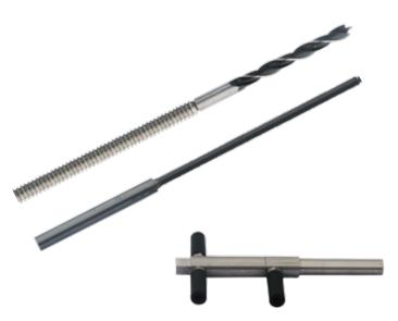
SDS setting tool for driving Lateral Restraint Ties into side of parallel floor joists, countersinking the remedial tie beneath the surface of the wall. Screws onto tie bar and fits into SDS drill. Driven into joists with hammer action disengaged.
