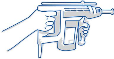
1. Drill hole to correct diameter and depth.
